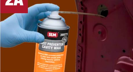
Clean surface with **SEM Solve** or **XXX Universal Surface Cleaner** where applicable. Remove cap from **Rust Preventer**, attach straw or **Rust Preventer Aero Wand**. Apply 1 – 2 coats.
