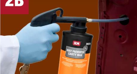
Clean surface with **SEM Solve** or **XXX Universal Surface Cleaner** where applicable. Shake bottle of **Rust Preventer** for 1 minute. Spray 1 – 2 coats at 35 – 45 psi.
