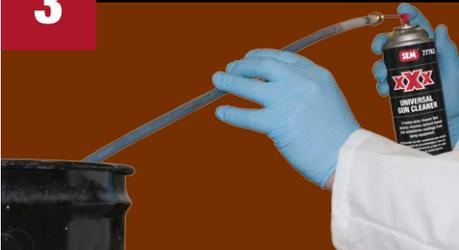
Clean **Aero Wand** by attaching the tip and wand to **XXX Gun Cleaner**.
